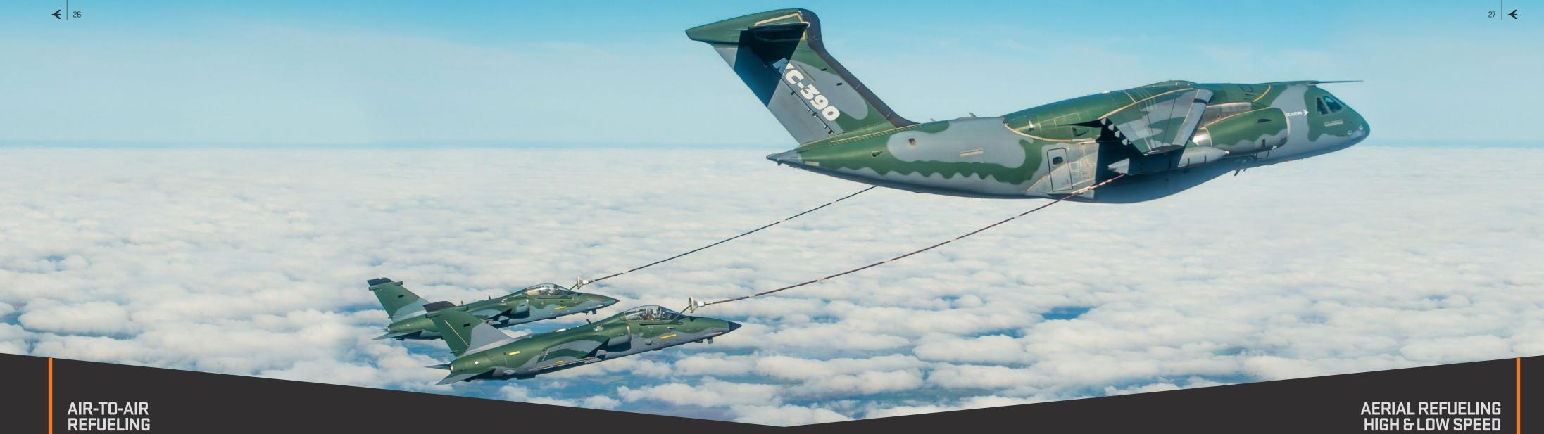
Day and night aerial refueling capability with observer windows and night vision cameras. The C-390 MILLENNIUM can be equipped with advanced refueling pods (Cobham 912E Series) that meet the high performance criteria of the aircraft providing a lightweight and efficient solution. Each pod provides fuel transfer up to 400 USgpm. Removable auxiliary fuel tanks can be installed in the fuselage to expand the aircraft fuel offload capacity or range performance.
